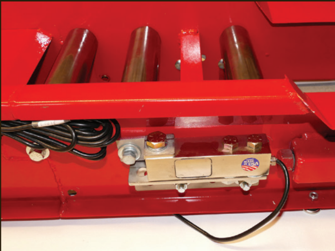
Conveyor scale with tube support rollers under flat belt. In this picture, the middle roller is connected to load cells.
