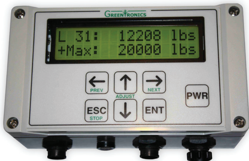
Controller with sealed keypad and bright display to navigate the menu system for configuration and calibration.
