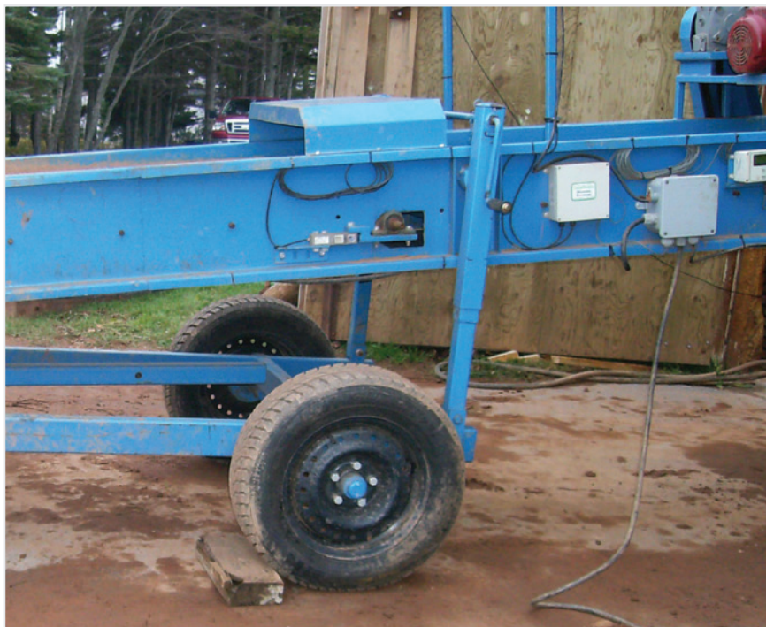
RiteWeight installed in portable conveyor with flat belt. A pair of load cells support one of the tube rollers. Any weight that passes over this area is measured and displayed.
