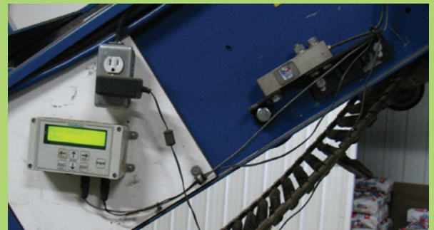
Controller with sealed keypad and bright display. Load cell mounted to exterior of frame and connected to support roller under the belted chain.
