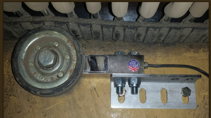
At left: Load cell mounted to support roller on Spudnik piler to the exterior of the frame. Above: Load cell mounted to the interior side of the frame on a Double L piler.
