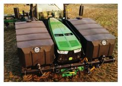
Improved visibility. The low-profile tank design improves front and side visibility from the cab.
