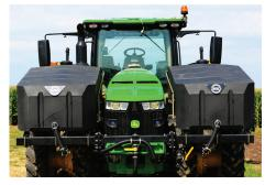
Narrow transport width. The tanks do not add to transport width. And, you still have access to the tractor's side panels for servicing.
